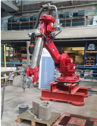
Fig. 3 Robotic arm employed for block printing (left).
