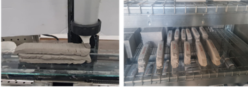
Fig. 1 Preparation of small-scale specimens: 2D extrusion of specimens (left), samples in the CO 2 chamber (right).
